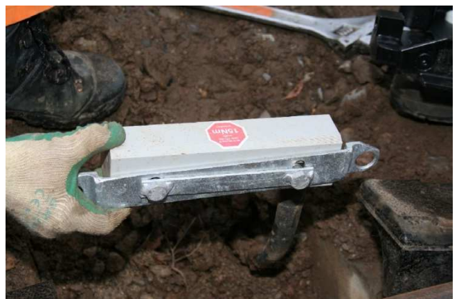
Axle counter on holding bracket.
