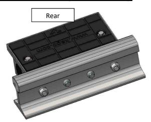
The KAGO Rail Attachment Box is form-closed to the rail and trafficable until 60 tons. It is self-supporting, this means the maximum carrying capacity is also guaranteed when used in lawn trace or other unfortified ground. The cable can be inserted from three sides and from underneath. Easy installation because of generous space inside the box. Cover screw connection with sliding blocks, i.e. replaceable when worn.
